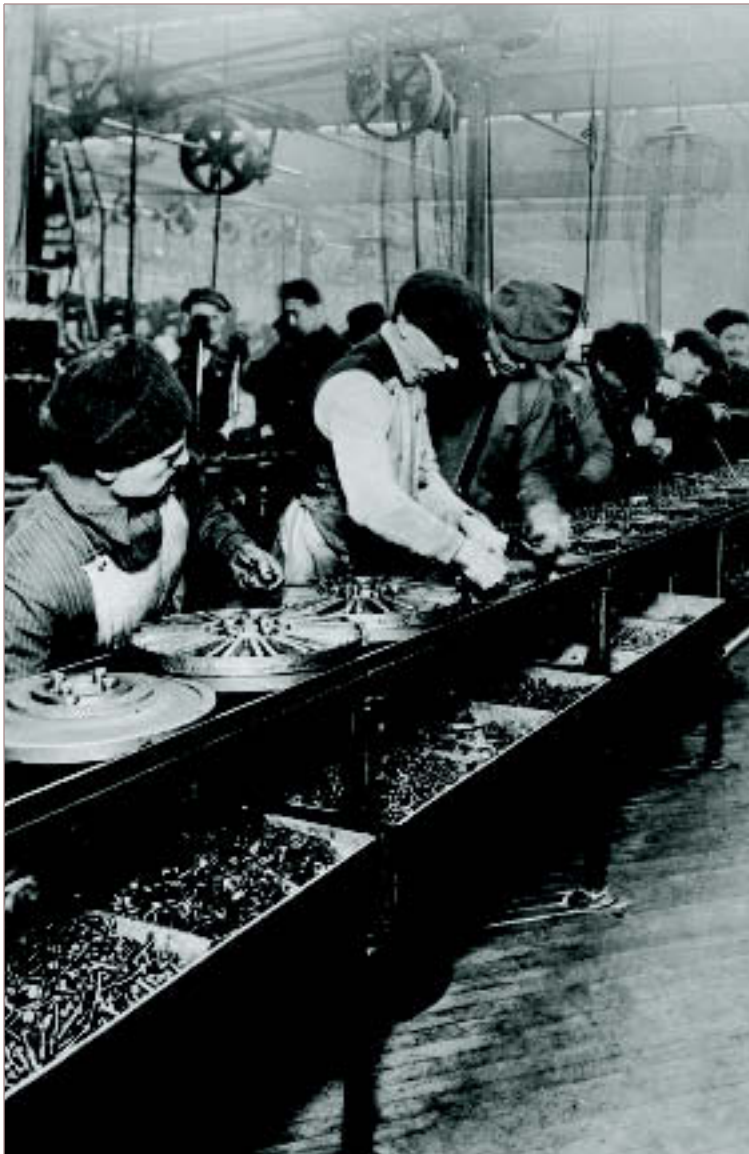
This flywheel assembly process at a Ford plant, circa 1913, was typical of the kind of repetitive task that defined the early Industrial Age.
